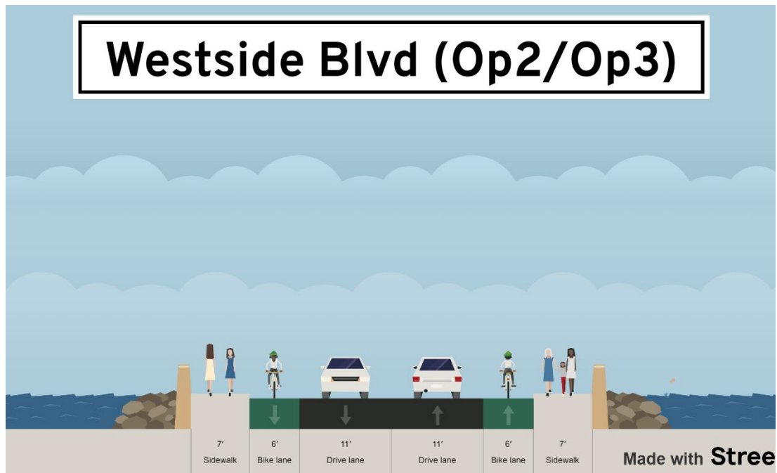
Figure 50 Westside Boulevard Proposed Cross-Section (Options 2 & 3)
